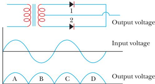
The contribution of output voltage from diode-2 is
