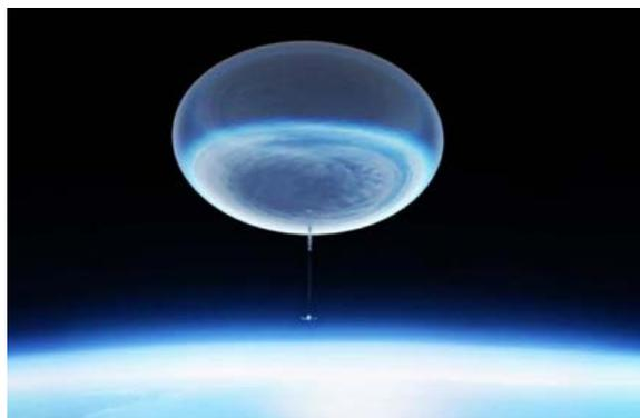
This mission will send a football stadium sized balloons into the stratosphere which will observe wavelengths of invisible light from the earth. The balloon has a telescope, sub systems, science instruments, electronic systems and cooling system. ASTHROS is Astrophysics Stratospheric Telescope for High Spectral Resolution Observation as Sub millimetre wavelengths.
