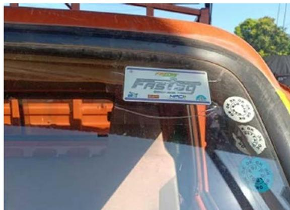
FASTags are the prepaid tags for automatic toll collection and work on Radio Frequency Identification technology. It will reduce the time of toll collection and will also ensure correct toll collection. These are usually pasted on the windscreen of the vehicles and rechargeable. The amount of toll is automatically deducted once these vehicles pass through the toll centre areas.
