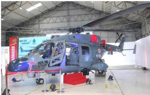
ALH Mk-III is an all-weather aircraft which will help Indian Navy to undertake medical evacuation of critical patients by air even during unfavourable weather conditions. Equipment can be installed in two-three hours to convert aircraft into an air ambulance.
